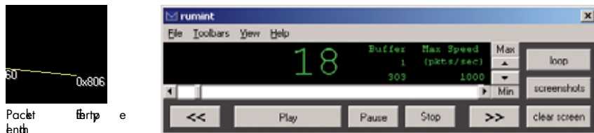
Figure 5-4: Using RUMINT's slider bar to locate the first ARP packet (left) at position 18 in the dataset (right)
