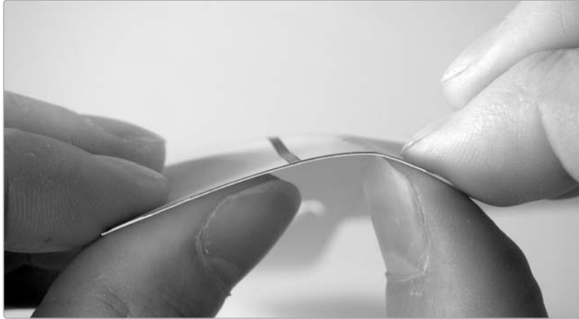
FIGURE 18-9: Making an easy airfoil by crimping the blade, as viewed from the edge of one boomerang arm; the leading edge is to the right
