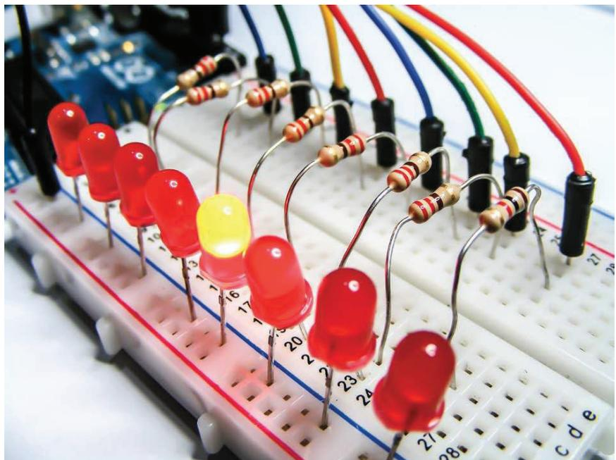
2. Connect the LEDs in sequence to Arduino digital pins 2–9, as shown in the following circuit diagram. Place a 220-ohm resistor between each LED and digital pin, ensuring that the resistors bridge the center divide in the breadboard.
