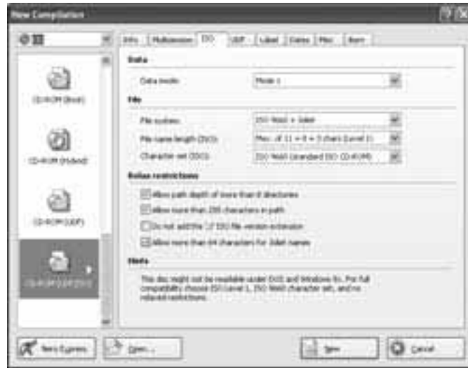
Figure 3-6: The ISO tab displays the optimum settings for burning an ISO disc for maximum compatibility.
