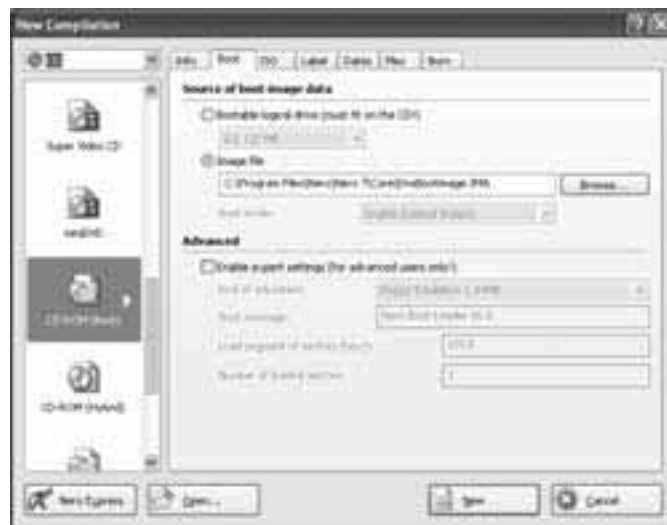
Figure 3-16: Nero provides an MS-DOS image file to boot from, but you can choose another operating system image file by clicking the Browse... button.
