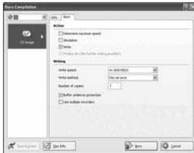
Figure 3-4: You can specify how many discs to burn and how fast to burn them with the Burn Compilation dialog box.
