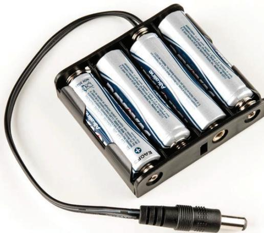
Unplug the USB cable from your computer, insert four AA batteries into your battery pack, and plug your portable battery pack into your Arduino, as shown in Figure 2-13. If your batteries are charged, you can move your project around or embed it directly into a model stoplight!
