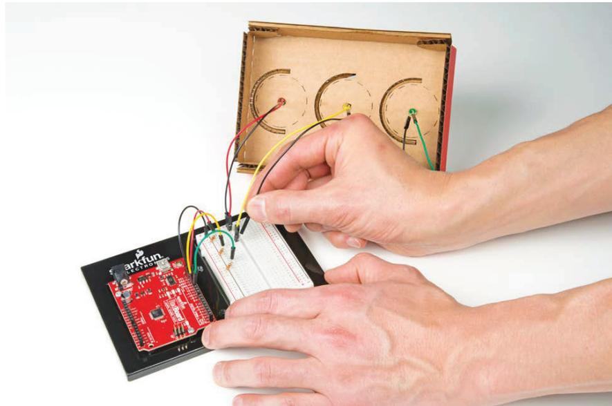
Check to make sure your connections work by plugging in the Arduino to your computer or to a battery pack. If one of the lights isn't working, try jiggling the connections or double-checking that the wires are plugged into the correct row on the breadboard.
