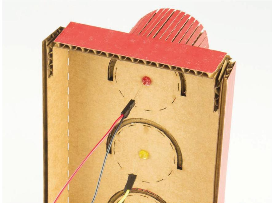
With the jumper wires connected to the LEDs, plug the male end into the breadboard in the same place where the LED came out, as shown in Figure 2-27. Again, pay attention to which LED goes where. If you don't remember, consult the original diagram in Figure 2-10.
