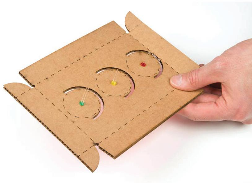
Next, bend the cardboard along the scored lines, as shown in Figure 2-19. Bend the vertical sides **1** toward the interior, and then do the same with the top and bottom sides **2** and the tabs **3**. (The sides and tabs are labeled in Figure 2-15.)
