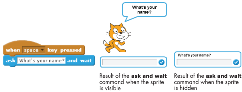
Figure 5-35: The ask and wait block may produce different outputs depending on whether the sprite that executes it is shown or hidden.
