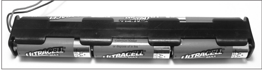
Figure 8-4: AA battery pack
