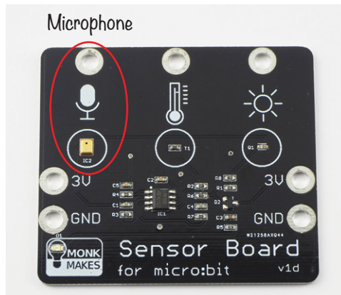
Figure 2-9: The Monk Makes Sensor for micro:bit microphone
