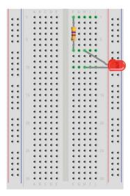
Now the positive pin of the LED is connected to the resistor—as shown in the circuit diagram—but the negative pin, like the upper pin of the resistor, isn't connected to anything.
