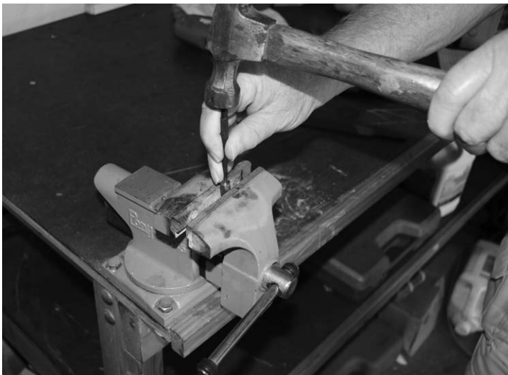
Figure 4-17: Clamp the shaft of the piece used as the bushing in a vise or pair of vise-grip pliers, and center punch a mark before drilling the hole. Get as close to the center as possible.
