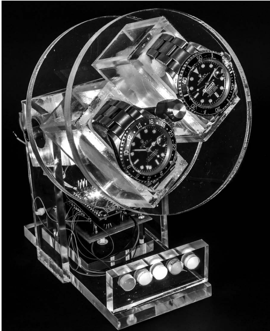
Figure 4-1: The finished Watch Winder. Unfortunately the black and white image doesn't do it justice: the brightly colored LEDs illuminate the device using the acrylic as a light guide to transport the various colored LEDs.
