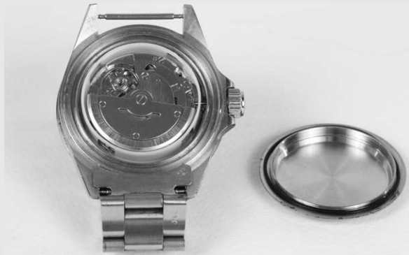
Figure 4-2: An automatic watch with the back removed, exposing the pendulum and the fulcrum (the screw in the center), which combine with a ratchet assembly to wind the watch's mainspring
