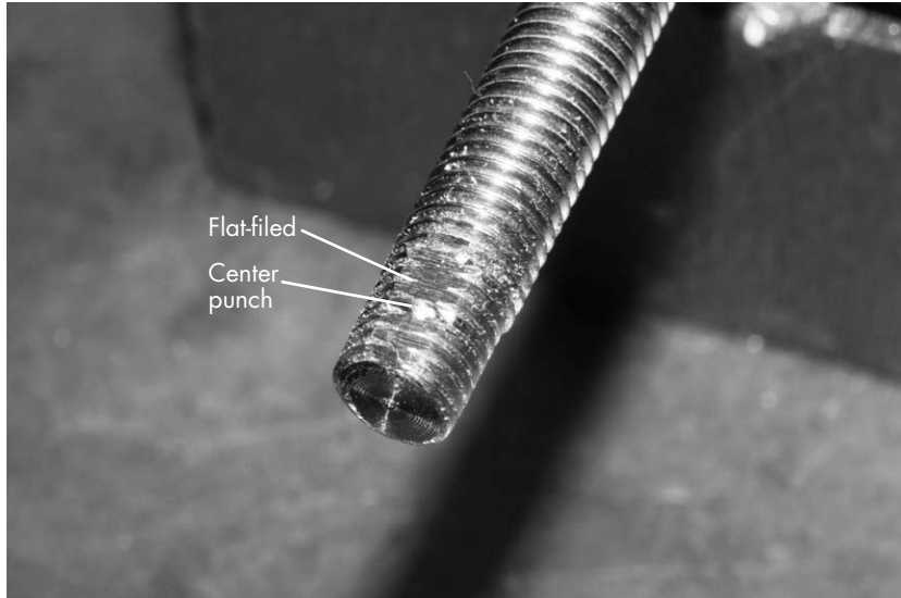
Figure 4-18: The easiest way to drill the holes in the threaded rod and bushing is to file a small flat on the shaft and center punch.
